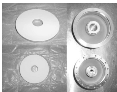
Fig. 3-2, 同軸平板型セラミクス (Tristan-type RF window with choke structure for STF) [1]
