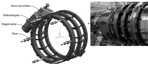
Fig. 3-31, Blade Tuner [33]
