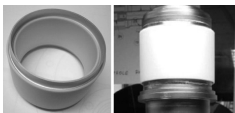
Fig. 3-3, 円筒型セラミクス (TTF-3 type cylindrical RF window for E-XFEL) [2]
