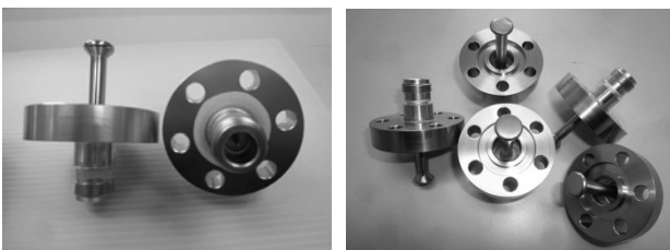
Fig. 3-30, RF feedthroughs for 1.3 GHz cERL injector 2-cell cavity at KEK [32]
