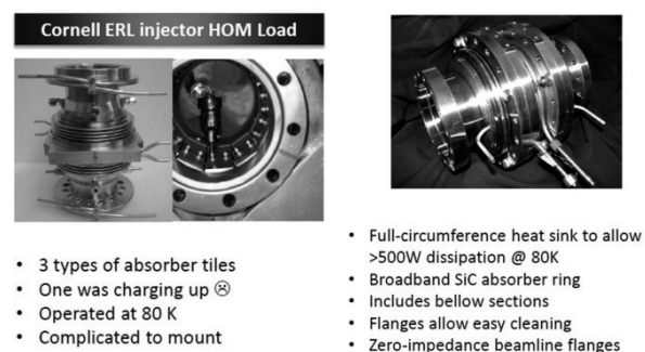
Fig. 3-27, HOM dampers for 1.3 GHz ERL Injector cavity (left [27]) and Main-Linac cavity (right [28]) at Cornell
