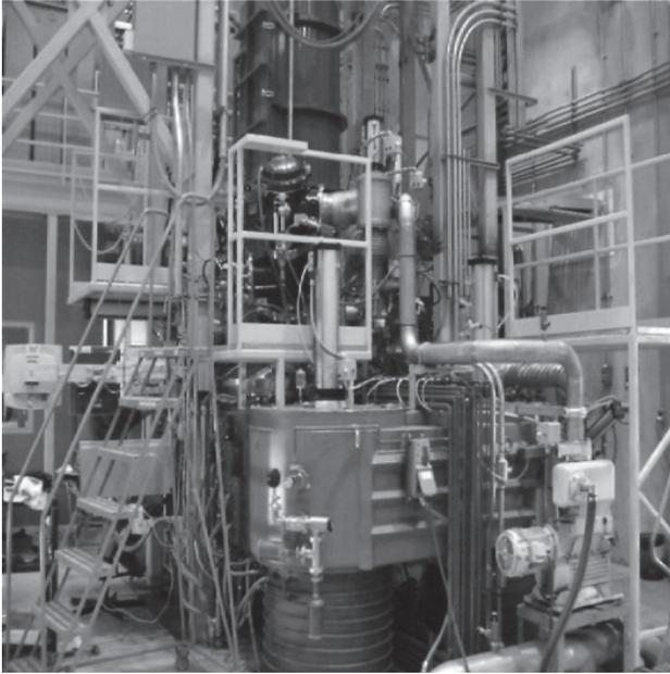
**Fig. 7 Electron beam melting furnace at ATI Wah Chang Company [9]**
