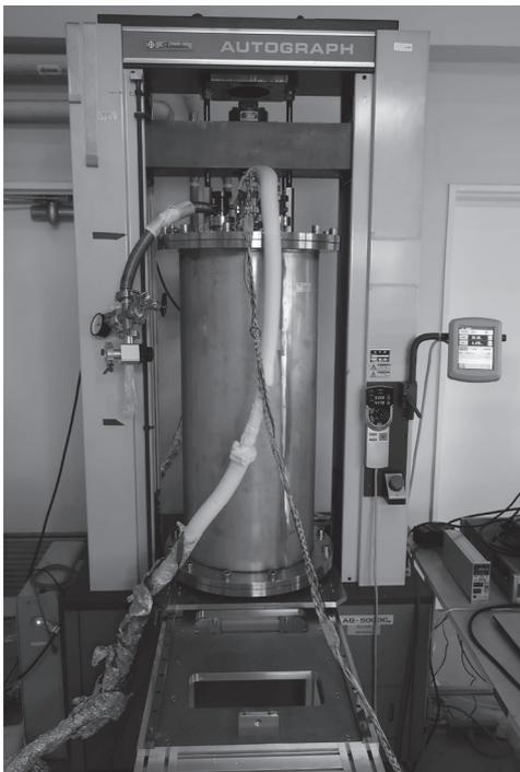
**Fig. 29 Schematic view of cryostat with tensile testing machine for liquid helium testing (top) [17]; Cryostat with tensile testing machine for liquid helium dipped tensile testing at KEK (below)**
