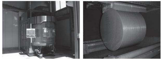
**Fig. 13 Frame format of multi-wire sawing (top); Multi-wire sawing machine and Slicing of Ingot (down) [19]**
