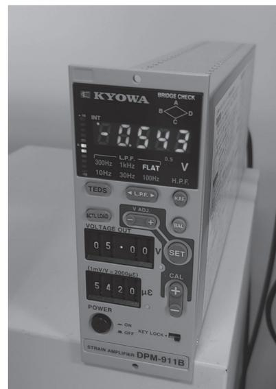
**Fig. 26 Kyowa® DPM- 911B strain amplifier**
