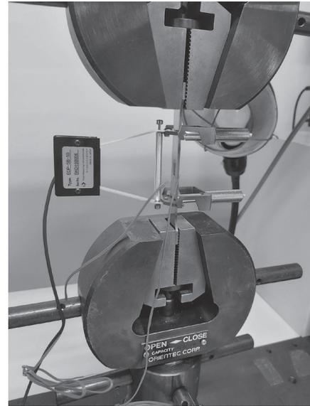
**Fig. 19 Clip-on type extensometer for room temperature tensile testing**
