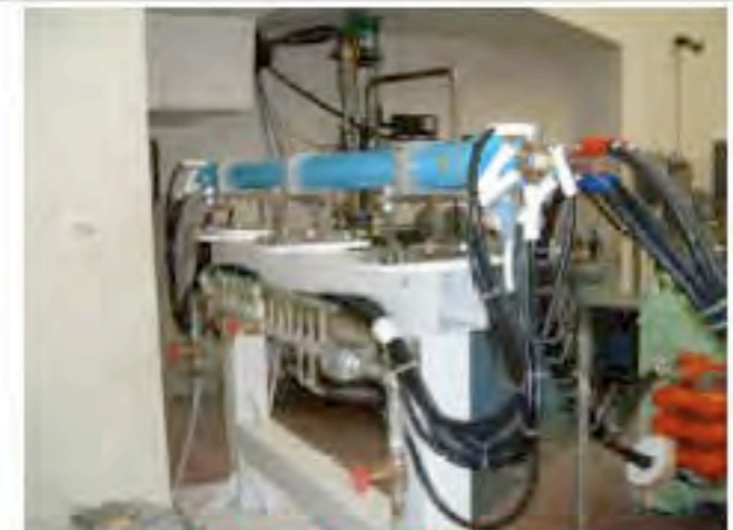
Sextupole Pulse Electro-Magnet
