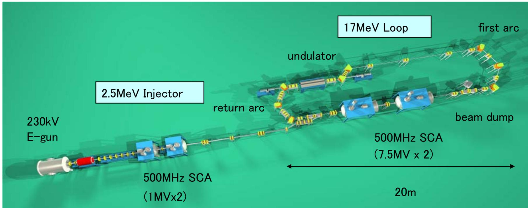
2.5 MeV injector consists of 230 keV thermionic cathode gun, 83 MHz sub harmonic buncher, and two single-cell 500 MHz SCAs.
