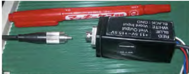
PMT: Hamamatsu H6780-02 with FC connector
