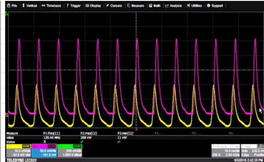
Pre amplifier characteristic @ 20A pump current
