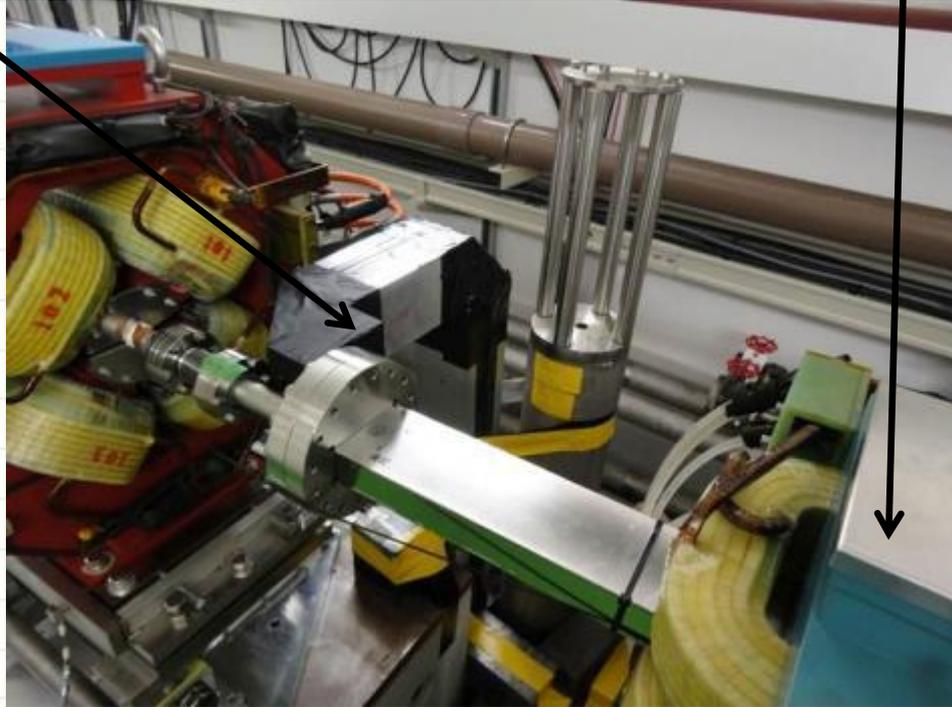
Cherenkov detector –  $\gamma$  converted to  $e^-/e^+$  pairs in lead, generate Cherenkov radiation in aerogel, guided to PMT below beam line.
