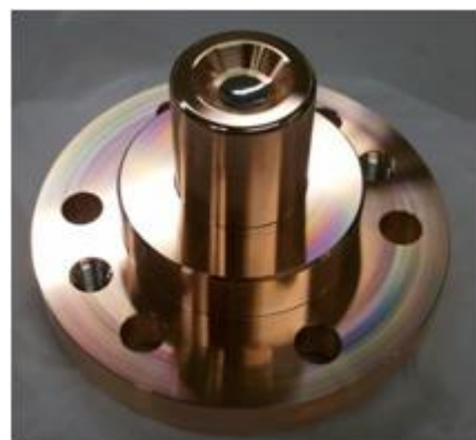
Fig. 13 Photograph of KEK-B photocathode
