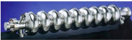
図.1 TESLA shape Superconducting Cavity [1]
