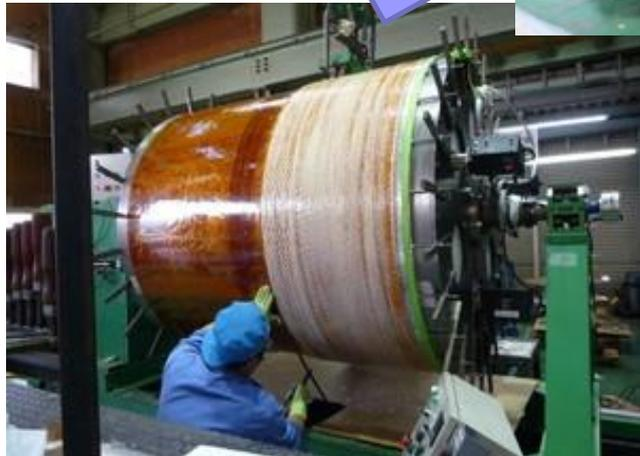
Wet winding with BT+Expoxy resin
