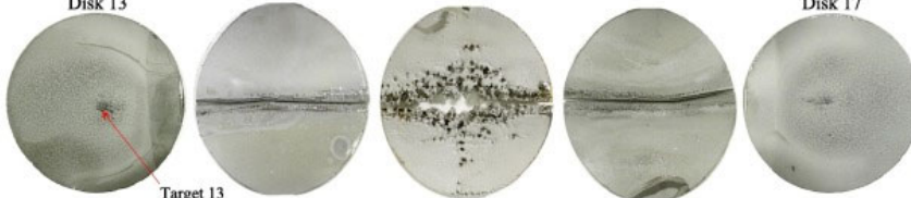
Target 13 leak location
