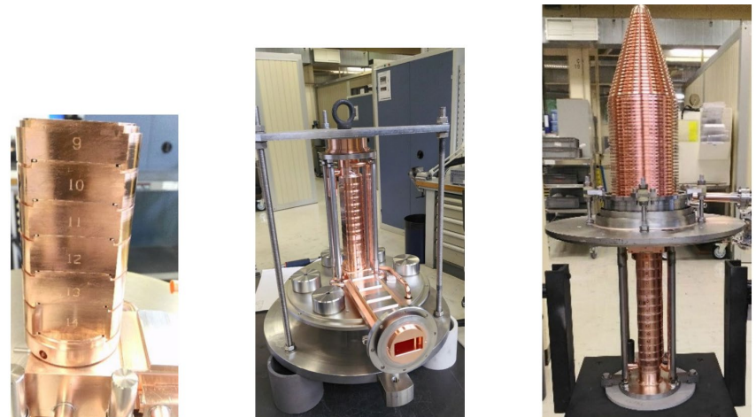
Fig. 11. Left: partial cavities assembly. Center: interaction line and output waveguide ready for brazing. Right: tube closed.
