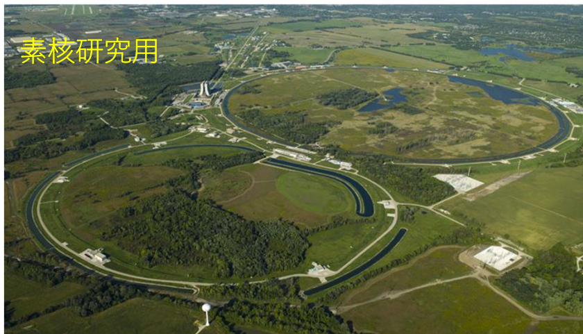
Main Injector, FNAL (Tevatronだった、USA) 120-GeV Synchrotron, 700 kW
